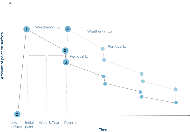
Figure 1. Schematic representation of Wear & Tear, removal and repaint cycle
